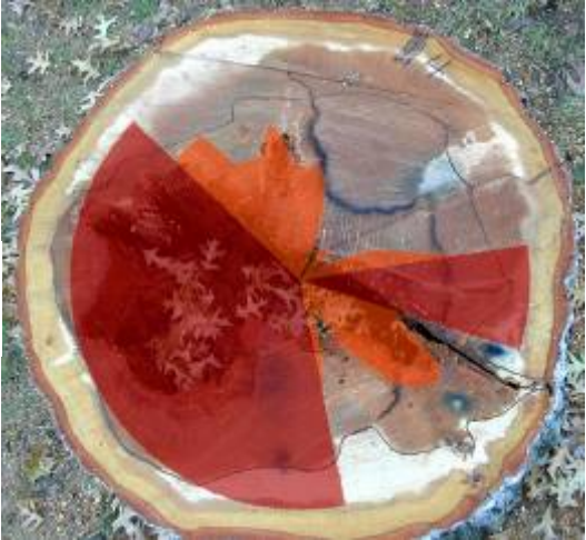
Overlay of Predicted Cross-Section onto Actual Cross-Section
