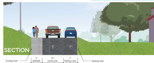
One-way traffic south of Navy Day Place with sidewalk on inside of the loop and on-street parking on the opposite side of the road. Traffic calming at key locations and additional green areas for potential landscaping are provided.
