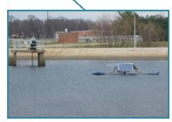
Fairfax County's Noman M. Cole, Jr. Pollution Control Plant replaced four standard 25 horsepower mixers with a solar mixer that is saving about \$40,000 a year in energy costs. (Source: Fairfax County)
