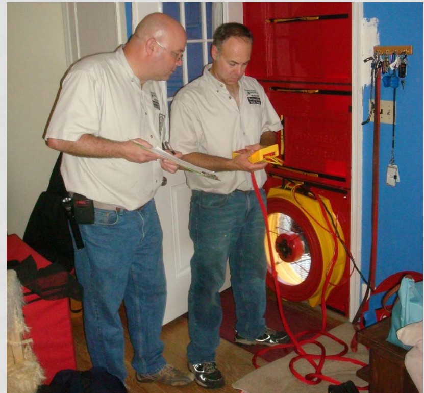
Energy experts set up blower door test to search for air leaks Photo Credit: Fairfax County
