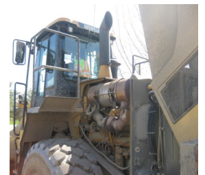
Front end loader owned by Reliable Contracting received diesel particulate filters which reduce fine particle emissions by approximately 90%.
