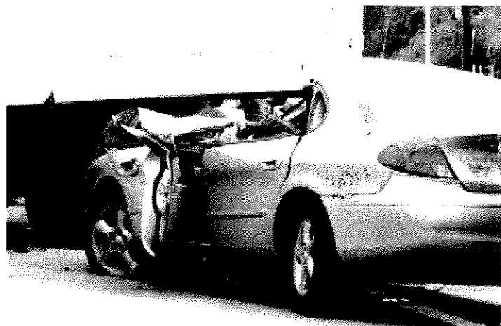
Car underrides beneath side or rear of trailer.
