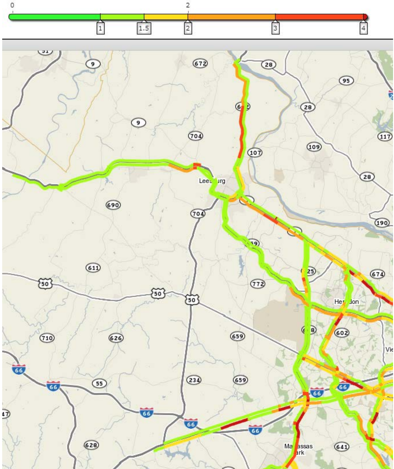
Figure B11: Planning Time Index on the non-Interstate NHS in Loudoun County, VA during Weekday 8:00-9:00 am, 2013
