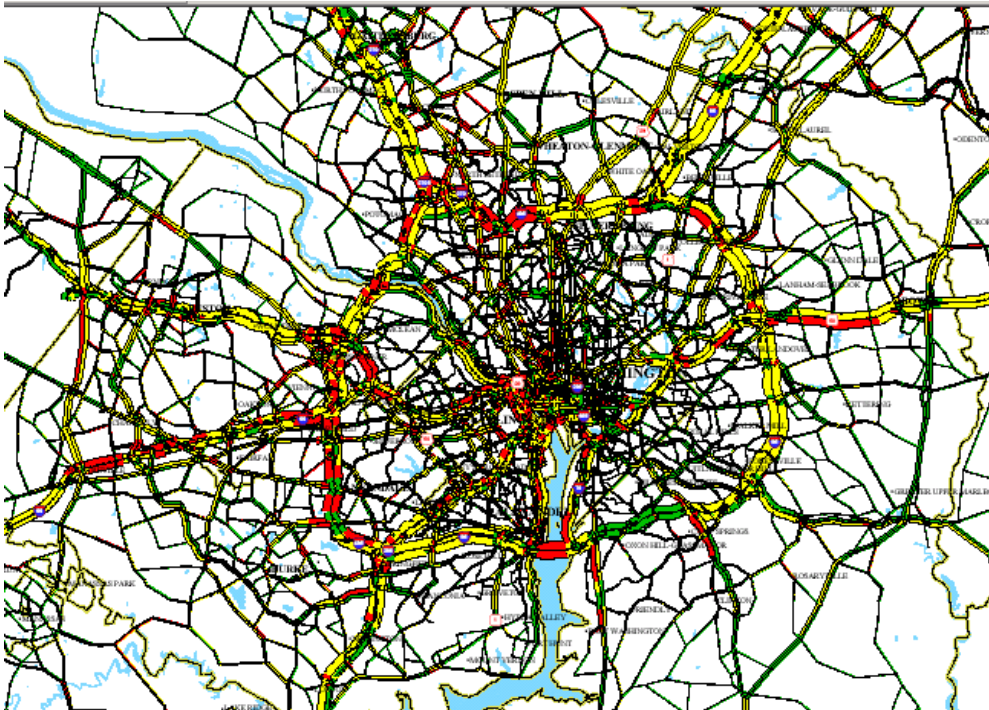
Figure A-II-3 With no demand management strategies or instructions to the public in place for the ice storm scenario, analysis shows much higher than normal demands on the region's roadway system.
