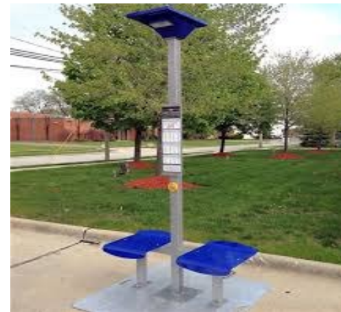
Enhanced bus stop post with attached seats and light (Lehigh and Northampton Transportation Authority)
