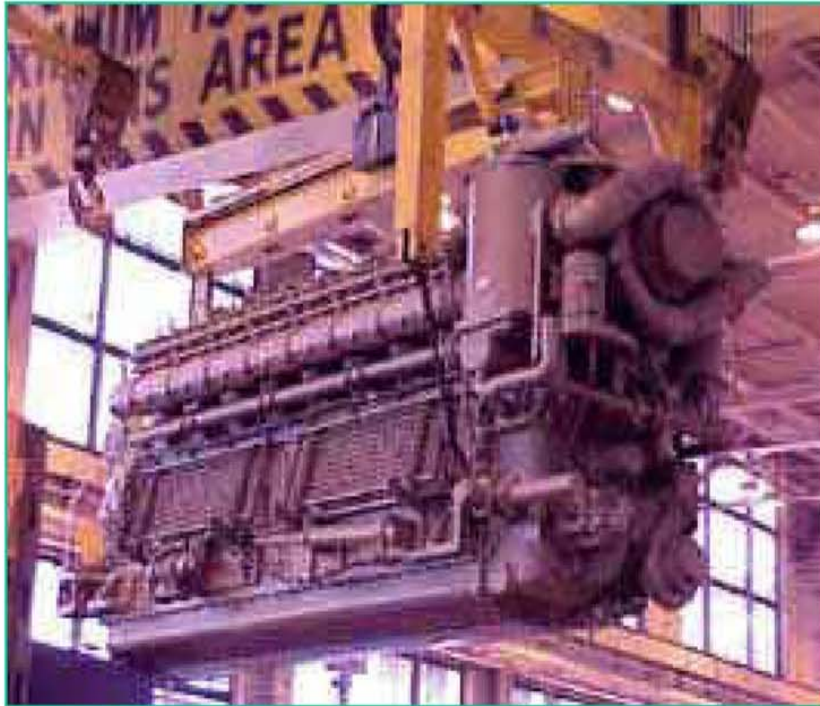
Typical 4400 HP locomotive diesel engine ... weighs 46,000 pounds
