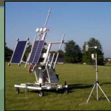
Solar Tracking Facility to Characterize Performance of Photovoltaic Cell Technologies
