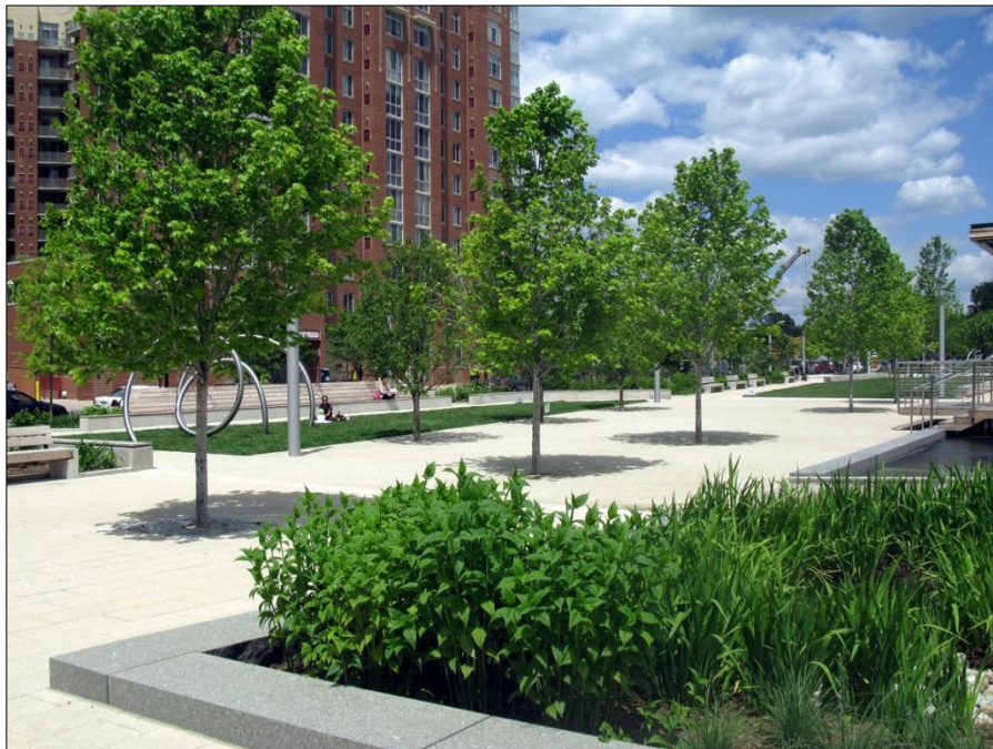
Figure 14: Washington Canal Park in Washington, D.C., uses rain gardens and permeable paving materials to capture rainfall and store it for reuse. Its light-colored surfaces and vegetation help reduce ambient air temperatures.
