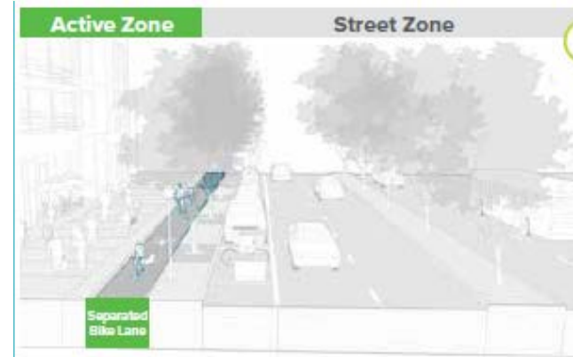
Figure 2-8. Separated Bike Lane
