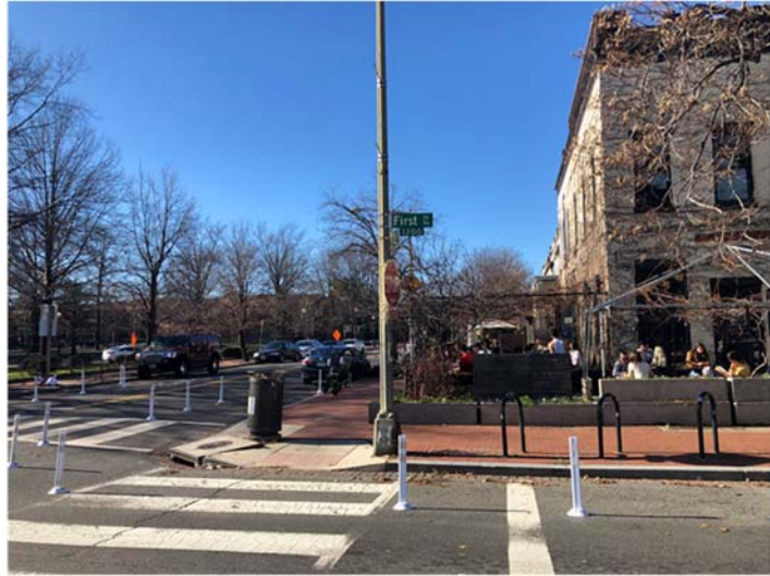
Figure 32: Flexpost Bulbouts/TPB/Michael Farrell
