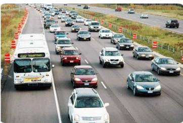
BOS is an arrangement by which buses providing public transportation service operate on designated highway shoulders, when safe and practical to do so, in order to circumvent peak traffic congestion.
