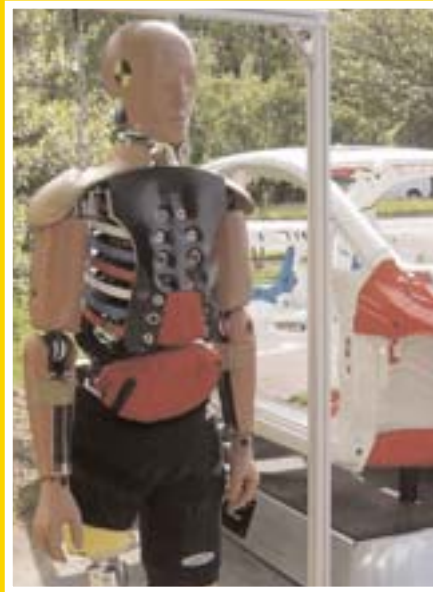
Honda created the first pedestrian crash test dummy in order to gain insight into engineering and design.
