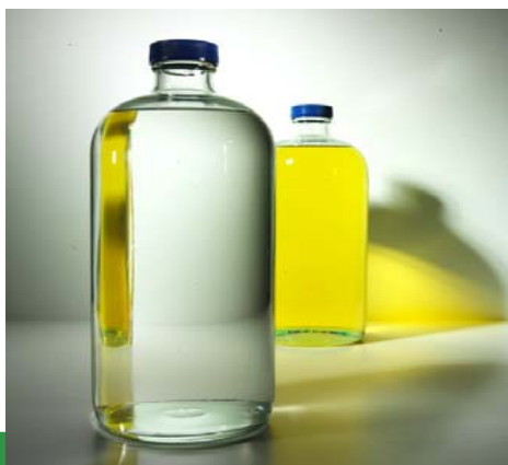
Amyris diesel fuel (clear) in front; petroleum diesel (yellow) in the back
