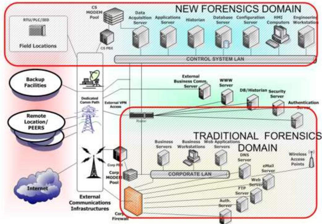
Figure 1. Control systems forensics domain and CSSP reference architecture.<sup>9</sup>
