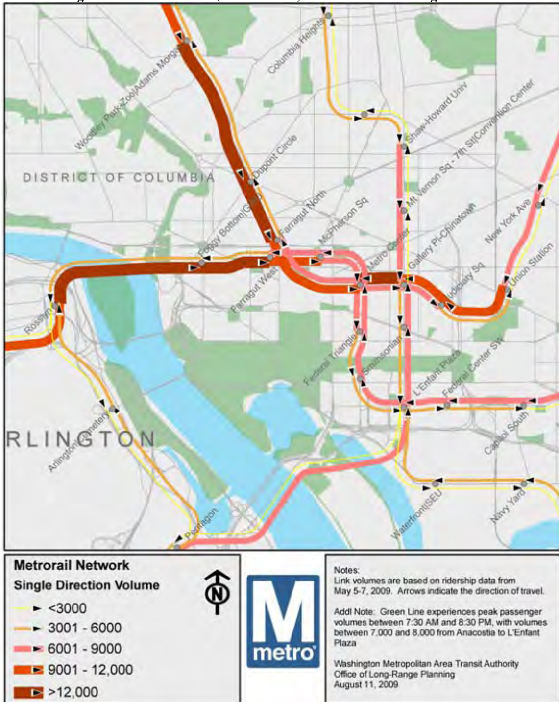
Figure 47: AM Peak Hour (8:00-9:00 AM) Metrorail Link Passenger Volumes
