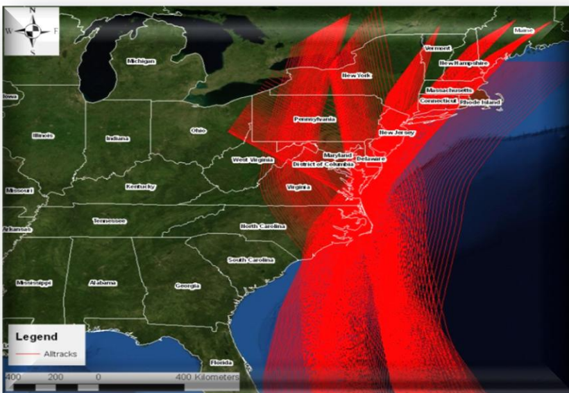
Figure 4. Over 500 hurricanes were simulated by FEMA in their recent floodplain re-mapping activities for the North Atlantic sea board. The RC-1701 project selected 17 of these storm tracks to use in this study. Ecological and shoreline data modeled under the five SLR scenarios were then used to re-parameterize the storms to generate the critical forcings (winds, waves, surge) for the regional assessment. These results were then handed-off to the nearshore and onshore modelers for further quantification of coastal storm impacts.
