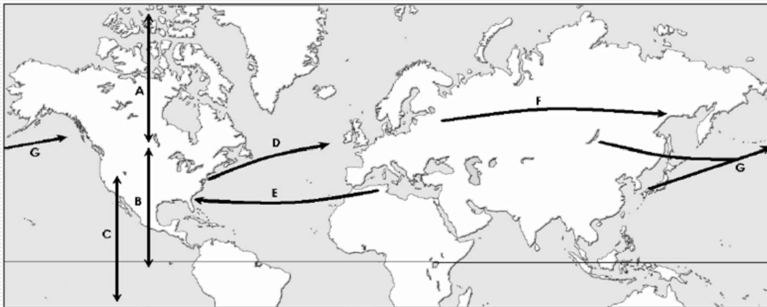
FIGURE 1.2 Major atmospheric transport pathways affecting North America. The general timescales of transport estimated by the committee from trajectory studies and other sources are: (A) Midlatitudes - Arctic exchange: 1-4 weeks. (B) Midlatitudes - Tropics exchange: 1-2 months. (C) Northern Hemisphere - Southern Hemisphere exchange: ~ 1 year. (D) North America to Western Europe: 3-13 days. (E) Northern Africa to North America: 1-2 weeks. (F) Eastern Europe to Asia: 1-2 weeks. (G) Eastern Asia to North America: 4-17 days. For (A), (B), and (C), transport occurs in both directions, depending on altitude.
