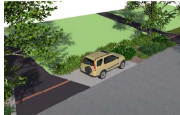
Bioswale, tree planters & permeable pavement: Fairfax Co.
