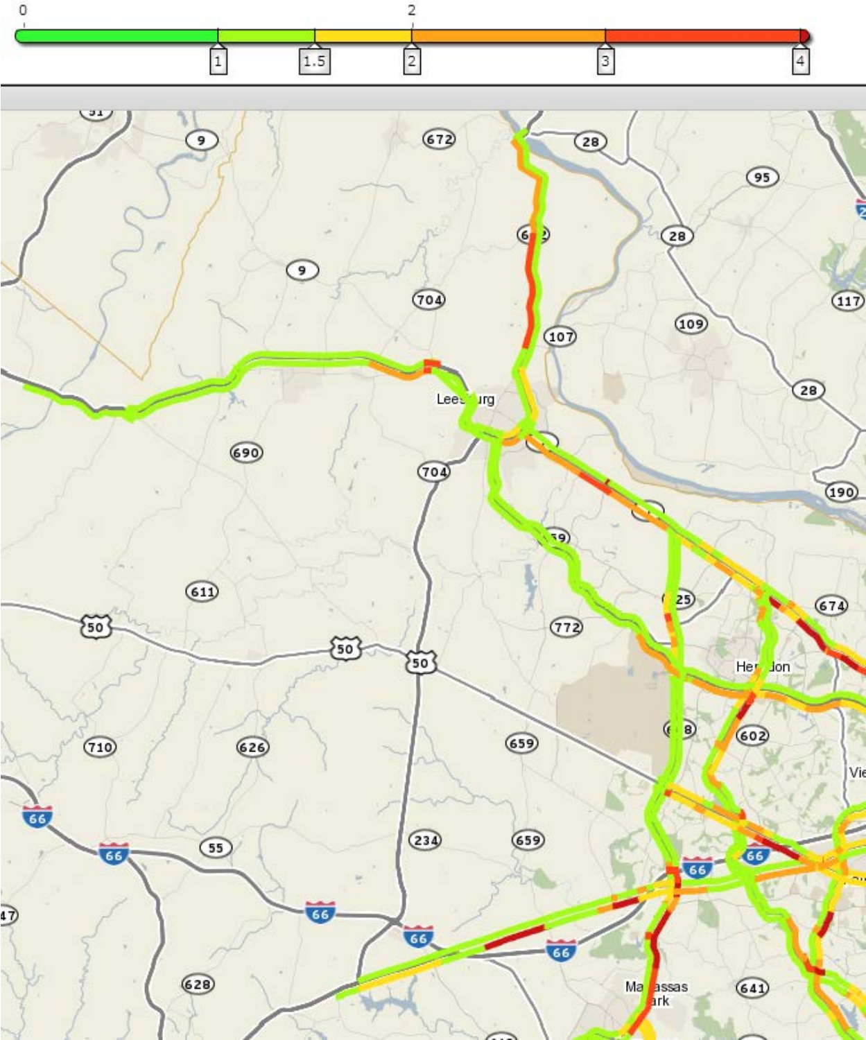
Figure B11: Planning Time Index on the non-Interstate NHS in Loudoun County, VA during Weekday 8:00-9:00 am, 2013
