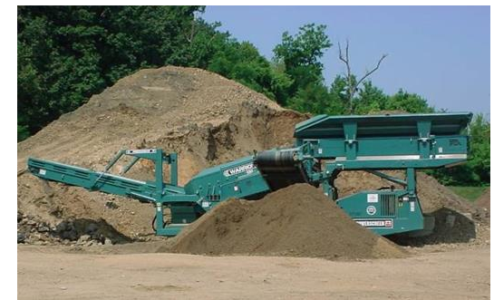
Dirt shaker-separates clean dirt from aggregate
