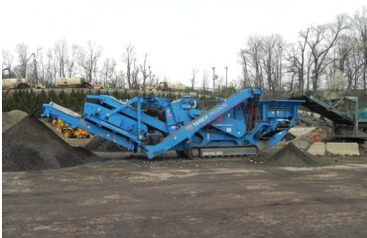
Crusher- concrete/asphalt/brick into aggregate
