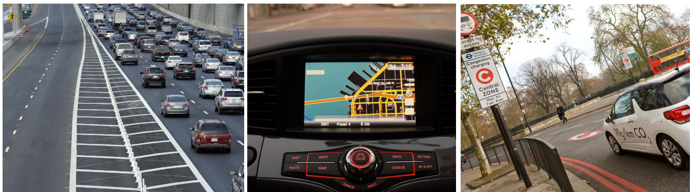
(Left) Scenario 1: Priced Lanes on All Major Highways. Drivers would have the option to pay a toll to travel in free-flowing lanes or drive in general purpose lanes free of charge.; (Center) Scenario 2: Pricing on All Roads and Streets. A fee would be applied based on distance traveled, time of day and road type.; (Right) Scenario 3: Priced Zones. Motorists would have to pay a fee to enter certain zones.
