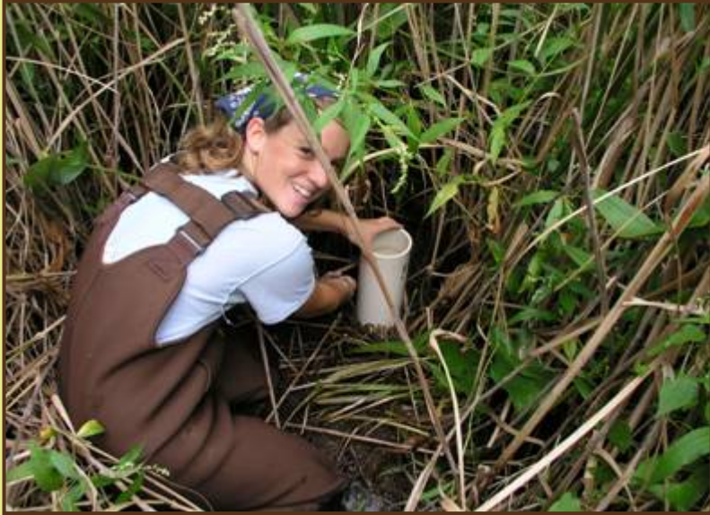
Cores taken by hand from high, mid and low marsh.
