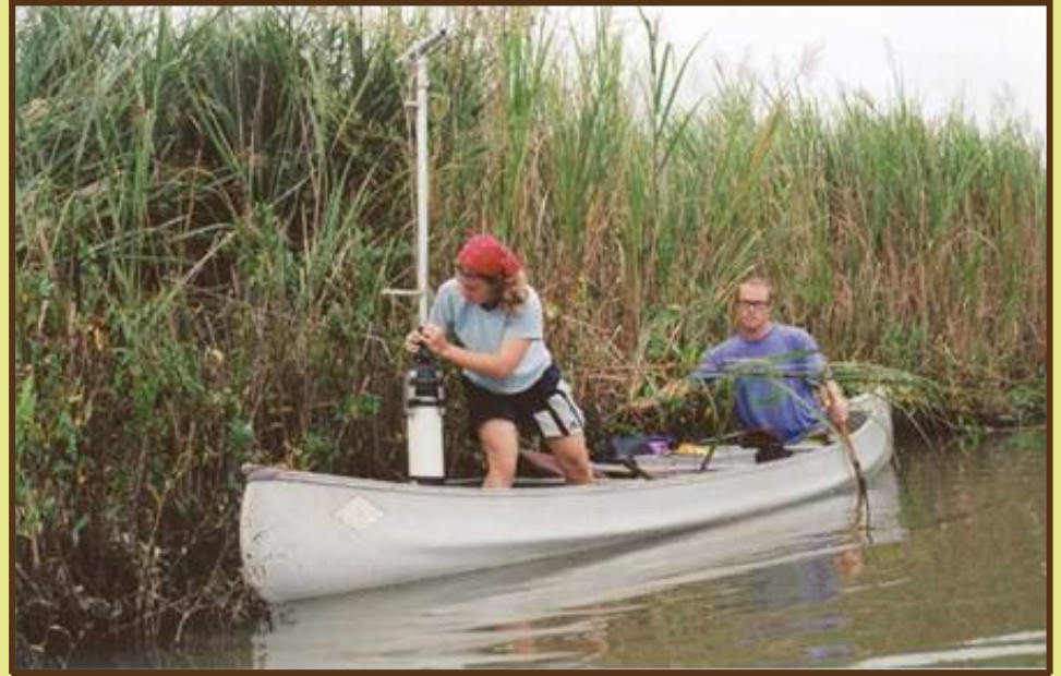
Marsh creek cores taken with a pole corer.
