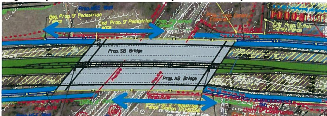
Figure 7: VDOT preliminary engineering plan with TDG recommendation for completing sidewalk network on both sides of the roadway
