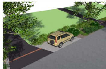
Bioswale, tree planters & permeable pavement: Fairfax Co.
