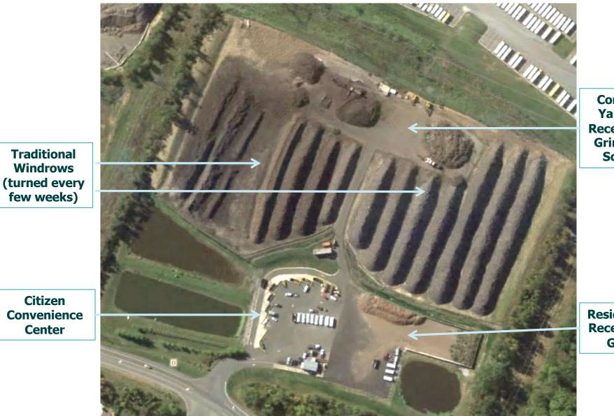
Commercial Yard Waste Receiving Pad: Grinding and Screening
