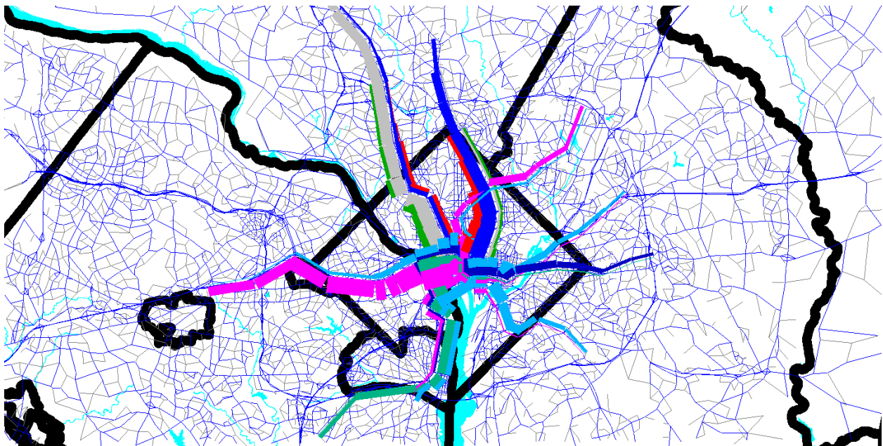
Figure 49 Using the pk_vol.dbf file in Cube Base as the transit layer: Only mode-3 (Metrorail) links turned on; using multi-bandwidth to represent transit loads (ab_vol): Metrorail system
