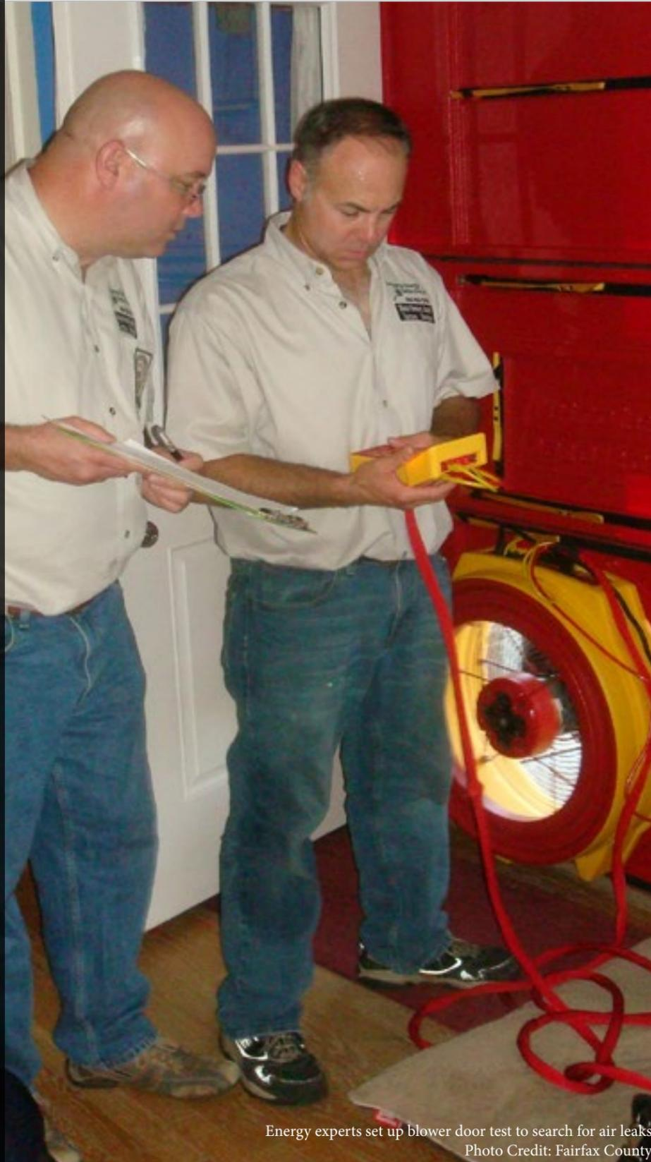
Energy experts set up blower door test to search for air leaks
