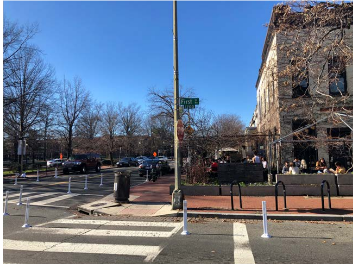
Figure 32: Flexpost Bulbouts/TPB/Michael Farrell
