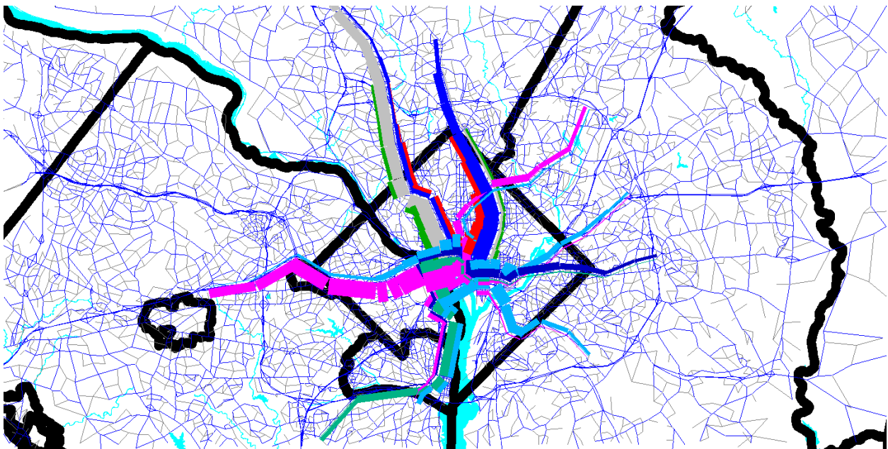
Figure 50 Using the pk_vol.dbf file in Cube Base as the transit layer: Only mode-3 (Metrorail) links turned on; using multi-bandwidth to represent transit loads (ab_vol): Metrorail system
