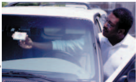
NEW TECHNOLOGIES HAVE MADE HOT LANES FEASIBLE. CUSTOMERS AFFIX TRANSPONDERS TO THEIR WINDSHIELDS. WHEN THEY USE THE HOT LANES, OVERHEAD ANTENNAS READ THE TRANSPONDERS AND DEDUCT TOLLS FROM PREVIOUSLY ESTABLISHED ACCOUNTS.
