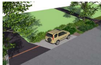
Bioswale, tree planters & permeable pavement: Fairfax Co.
