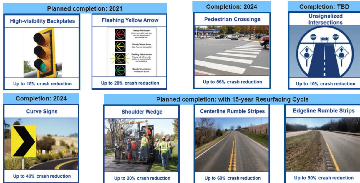
Figure 8 VDOT Systemic Safety Countermeasures and Schedules 1
