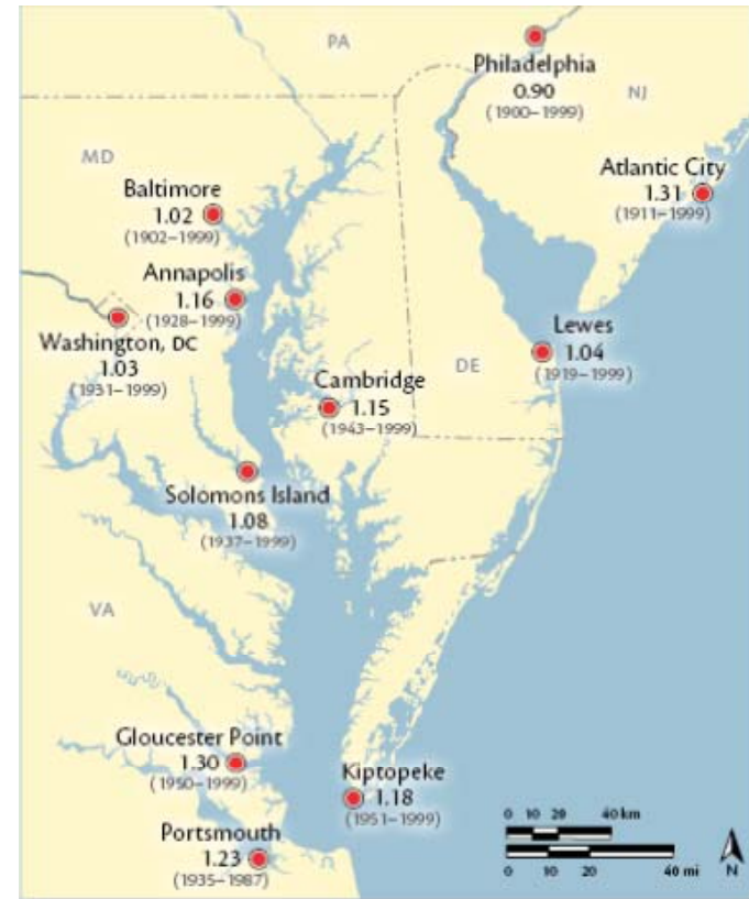
Rates of SLR (ft/century) for the Chesapeake and Delaware Bays Region. Data from tide gages and data record shown in parenthesis. Source: The Maryland Commission Climate Change
