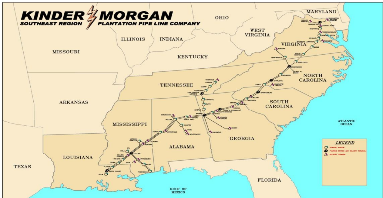
Figure 8-13. Plantation Pipeline Owned by Kinder Morgan
