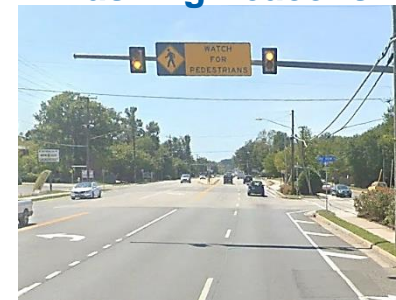
Warning Sign with Flashing Beacons
