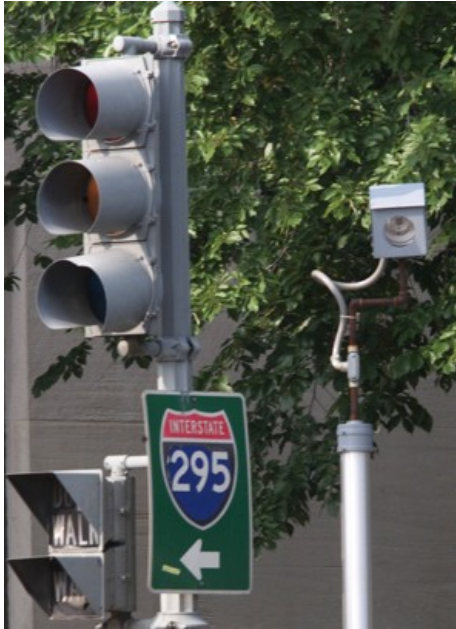
A camera is placed near a traffic light for drivers who run red lights on Constitution Avenue. (Mark Wilson - Getty Images)
