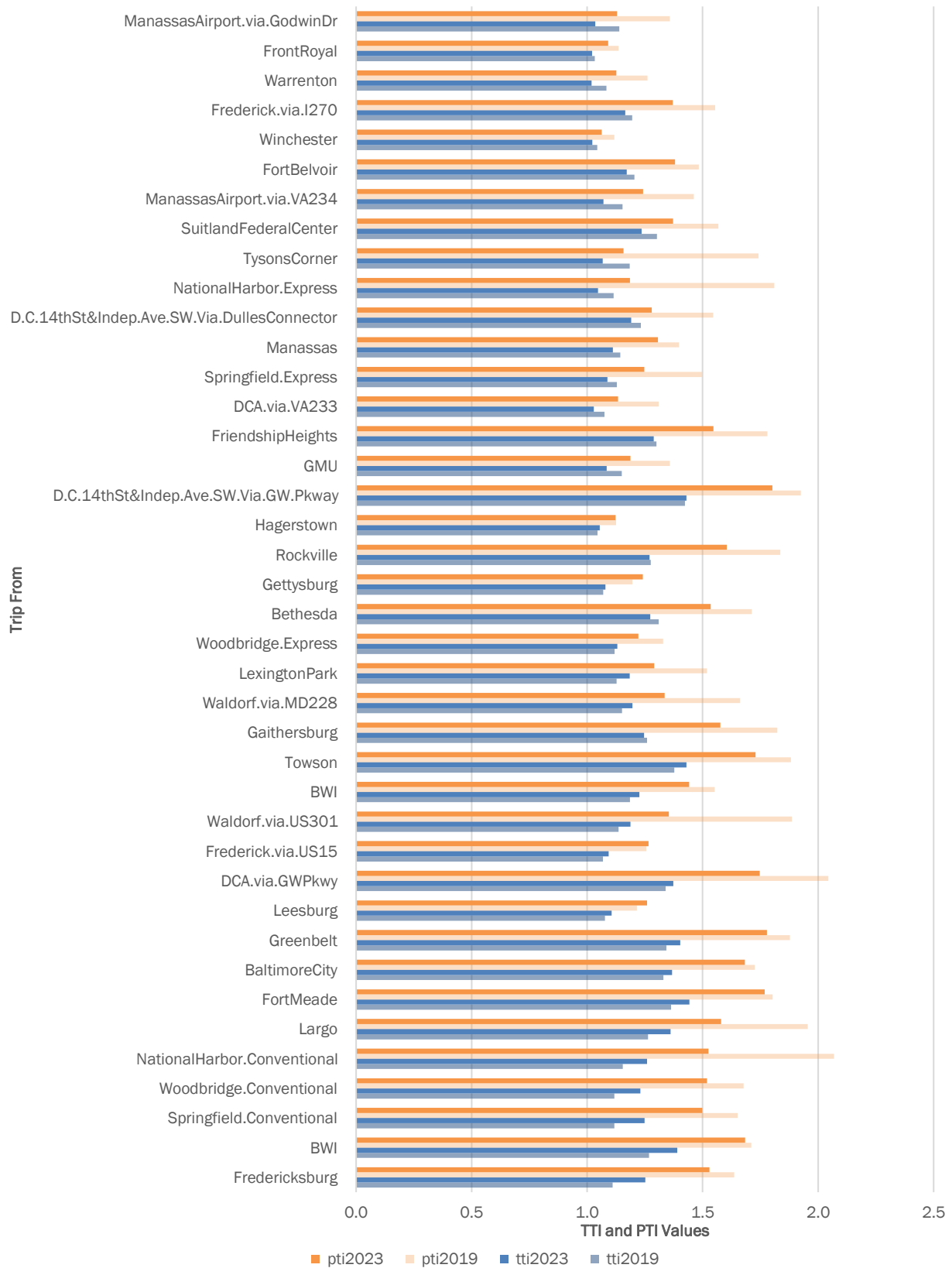
Figure 24. IAD 3 PM – 7 PM Weekday Travel Time Index and Planning Time Index Aggregate Values
