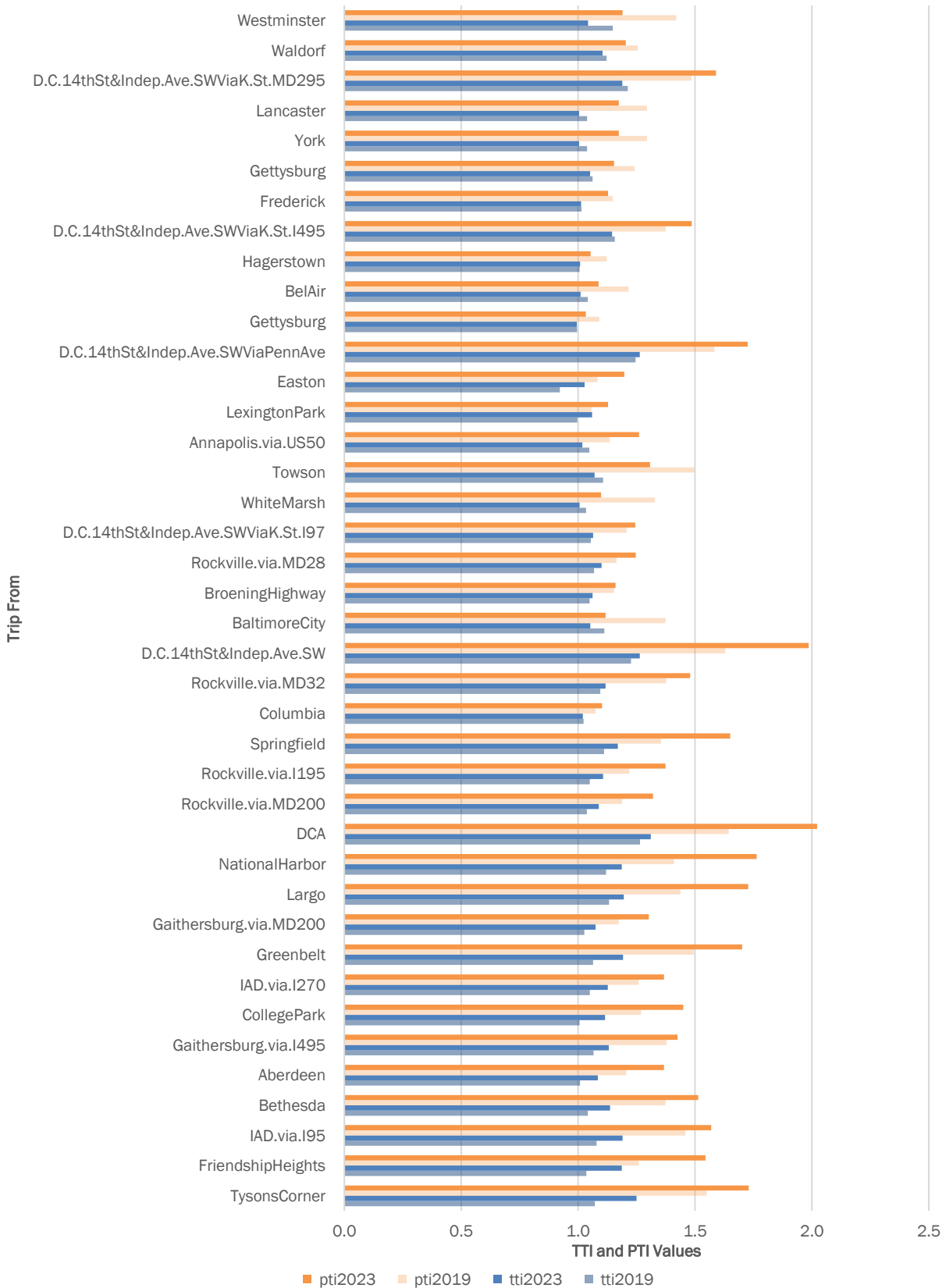
Figure 11. BWI 9 AM – 3 PM Weekday Travel Time Index and Planning Time Index Aggregate Values
