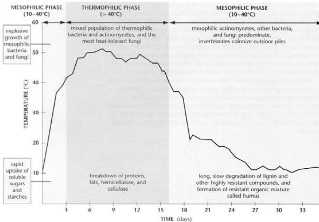
You can map the progress of thermophilic composting by taking periodic temperature measurements and charting a “temperature profile” [Figure 2.6].
