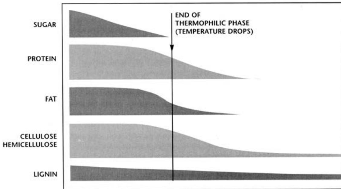
**figure 2.8: the effects of turning on composting temperature**
