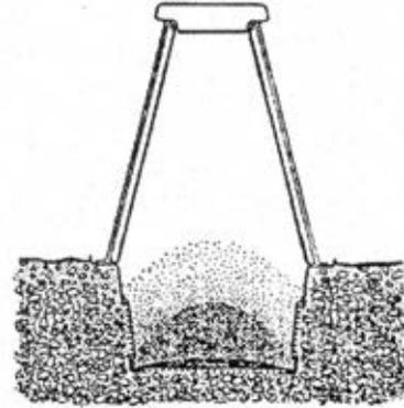
Note: In order to prevent flooding and the subsequent exposure of leachate to the air (which can be smelly!), a digester should be placed in well-drained soil.
