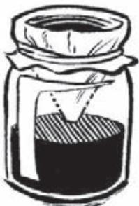
**1. Bottle fly trap** (right). Cut a small plastic water or soda bottle in half. Fill the bottom half with some apple cider or beer and a drop of detergent. Turn the top half upside down and place it into the bottom half so that the neck forms a funnel. Secure the two halves with tape.
