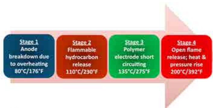
Figure 7 - Thermal Runaway Process - Source: E-cell Secure, LLC (2020)
