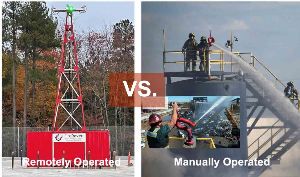
Figure 12 - Remotely operated Fire Rover Water Tower versus Manually Operated Water Tower. As you can see, one option requires humans to be proximate to a potential fire, whereas the other is remotely operated and does not.
