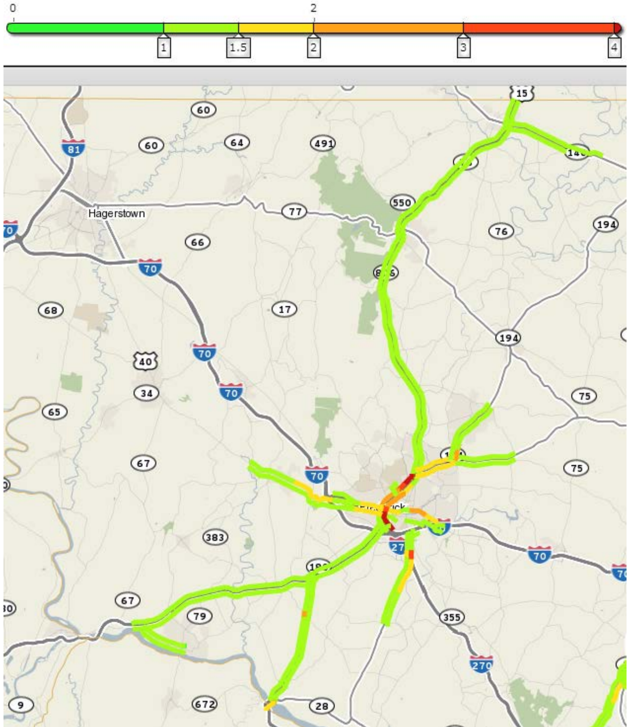
Figure B6: Planning Time Index on the non-Interstate NHS in Frederick County, MD during Weekday 5:00-6:00 pm, 2013
