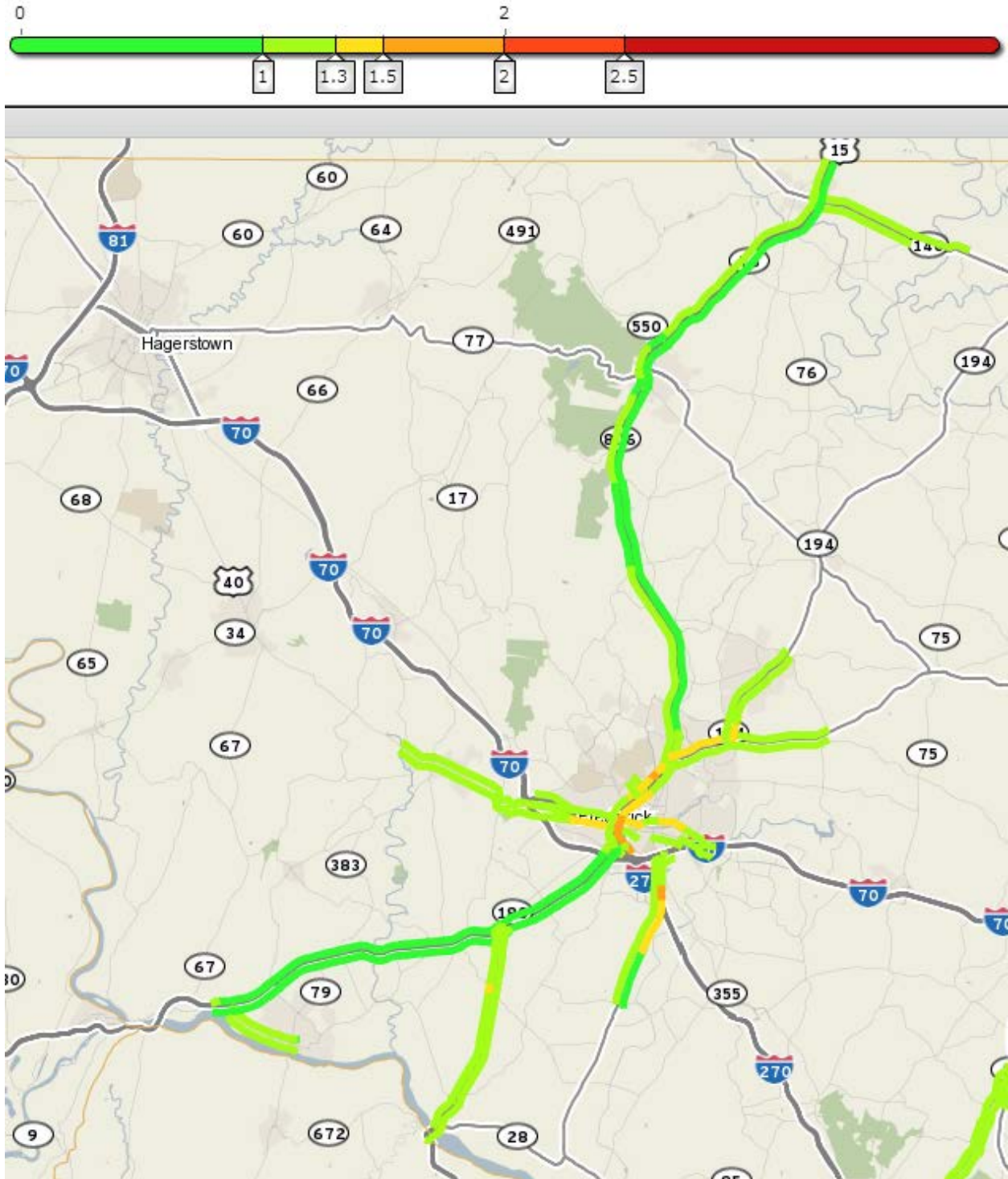
Figure A6: Travel Time Index on the Non-Interstate NHS in Frederick County, MD during Weekday 5:00-6:00 pm, 2013
