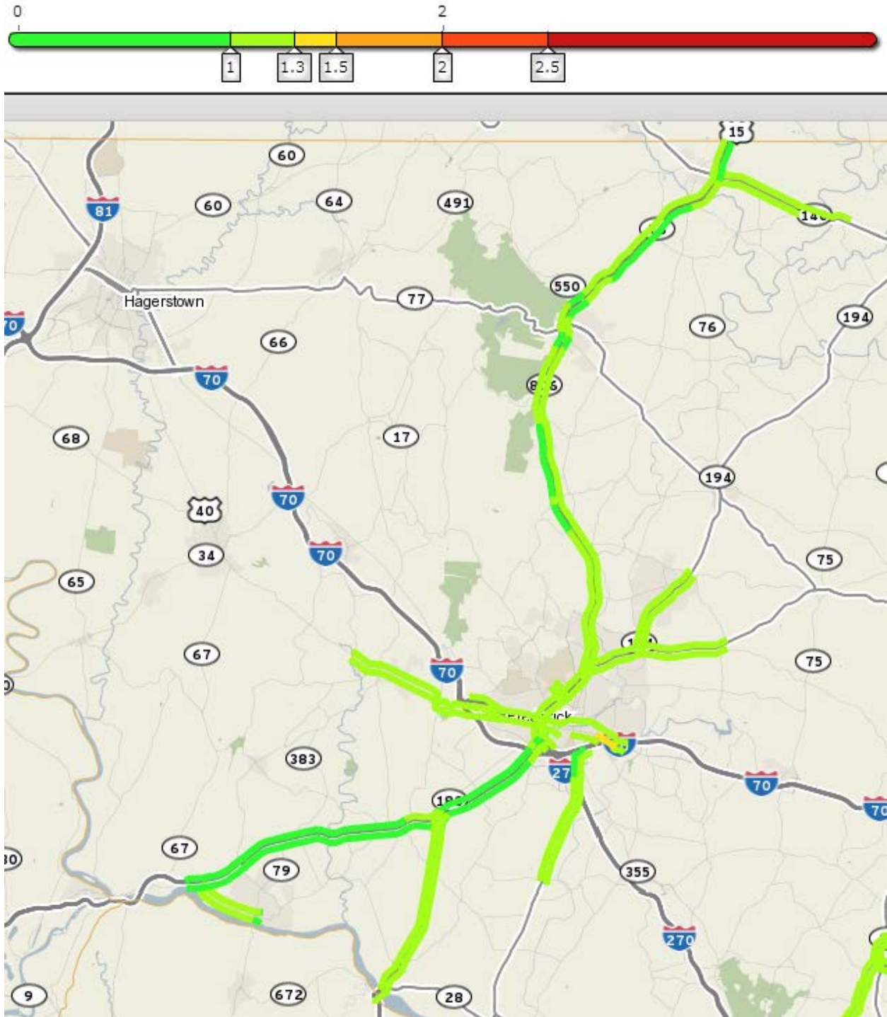
Figure A5: Travel Time Index on the Non-Interstate NHS in Frederick County, MD during Weekday 8:00-9:00 am, 2013
