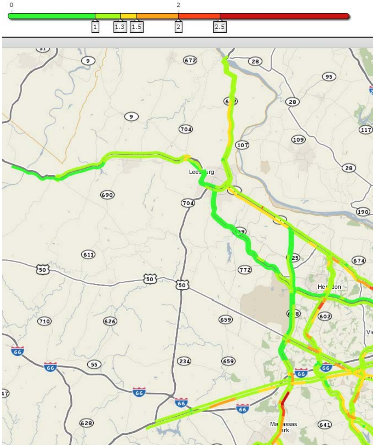
Figure A11: Travel Time Index on the Non-Interstate NHS in Loudoun County, VA during Weekday 8:00-9:00 am, 2013
