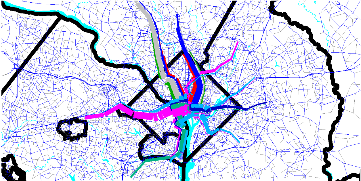
Figure 24 Using the pk_vol.dbf file in Cube Base as the transit layer: Only mode-3 (Metrorail) links turned on; using multi-bandwidth to represent transit loads (ab_vol): Metrorail system
