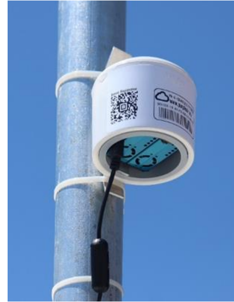
The image above is a purple air sensor. It measures particulate matter.
