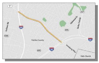
9. Construct Collector-Distributor Roads Parallel to Dulles Toll Road between VA 684, Spring Hill Rd. and VA 828, Wiehle Ave.
