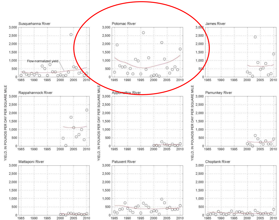
Figure 5. Estimated annual yields of suspended sediment at the nine U.S. Geological Survey River Input Monitoring (RIM) stations, Maryland and Virginia. (Trends in yield are computed on the basis of differences in flow-normalized yields over a given period of time; axes are scaled identically to permit comparisons of watershed yields over time. Modified from Moyer and others, 2012, fig. 22). http://chesapeake.usgs.gov/
