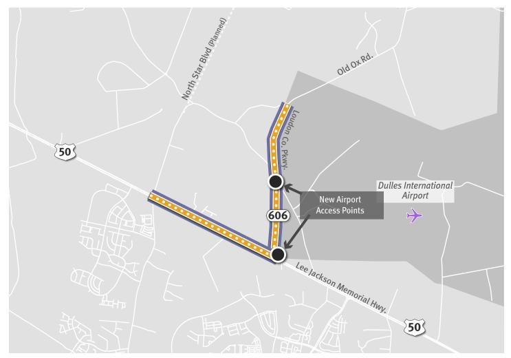
Construct two Airport Express Lanes in the median of US 50 between Northstar Boulevard/Bi-County Parkway and VA 606, Loudoun County Parkway, at New Dulles Airport Access. Upgrade US 50 within the same limits to a limited access facility and widen from 4 to 8 lanes. Upgrade VA 606, Loudoun County Parkway, between US 50 and VA 607 to a limited access facility and widen from 4 to 6 lanes.
