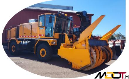
3,500 tons of snow removal capacity per hour
